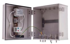
The AccelTex Solutions Heated PoE enclosure allows an access point to be installed in an outdoor or other temperature-limiting environment. The heater and AP are powered by a single PoE cable run from the network switch. The enclosure ships ready for an AP and external antenna installation.
